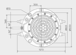
Discharge Pipework B:40/50mm V:50mm
