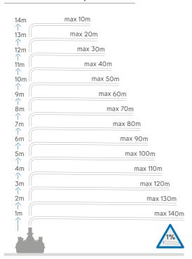
Max pumping height 16m at 0 flow rate
