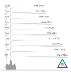
Max pumping height 13m at 0 flow rate
